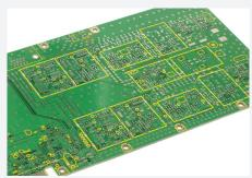
Separate certain sections or circuits on the PCB. For example, keep noisy power supply circuitry away from sensitive RF circuitry.
